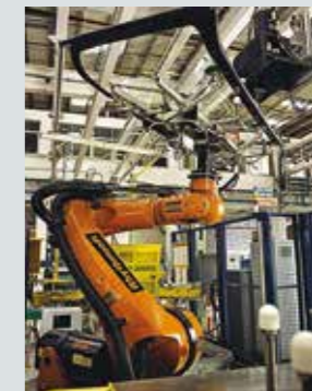
A robot affixes the windshield on a truck with high precision.
