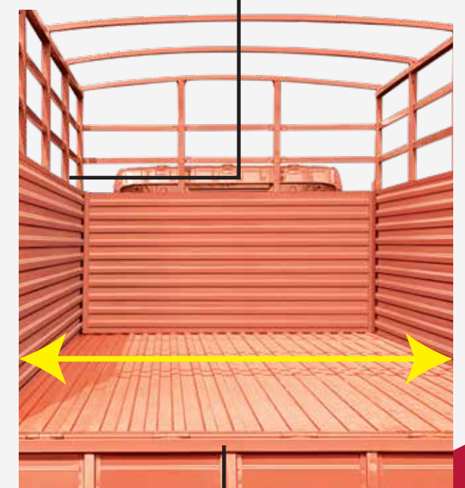
Five Hinges on Tail Panel for added strength
