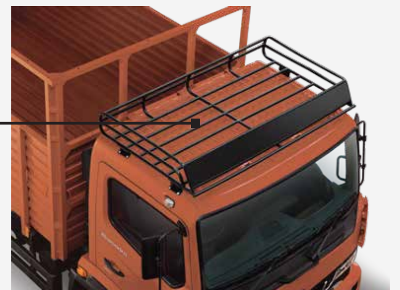
High Strength Low Alloy (with Grade 420 Panels) needs no extra reinforcement
