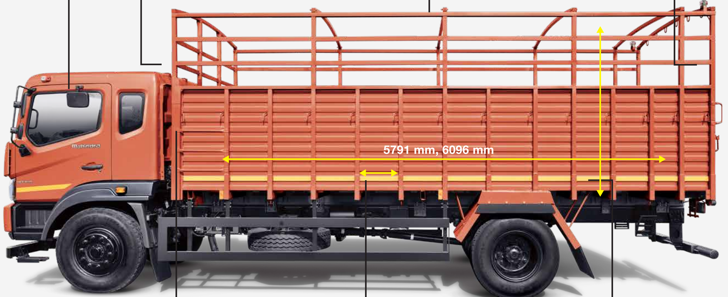
High Strength Low Alloy (with Grade 420 Panels) needs no extra reinforcement
