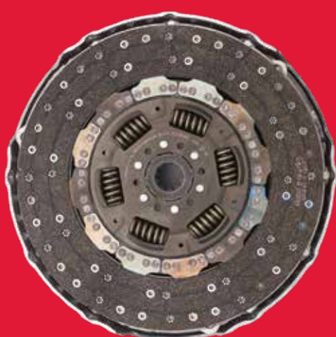
362 mm Diameter Organic Clutch
