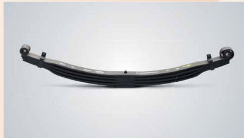
Softer Parabolic Suspension with Rubber Tips for Best-In-Class Comfort to Absorb Bumps and Jerks
