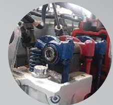
Hydraulic Lash Adjuster No tappet setting required
