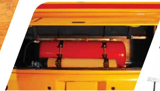
Water Tank And Nitrogen Tank
