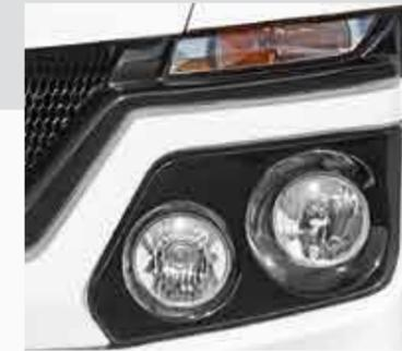
**Twin Round Headlamps** provide better light spread at night with both upper and dipper light arrangement for better light vision & safer night driving for drivers
