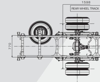
**Side Spare Tyre Mounting** provides easy opening of spare tyre just by jack rod arrangement, so there's no need for helpers or conductors to lay down under the bus to remove the tyre.
