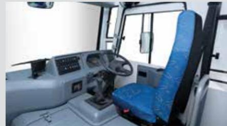
**4-way Adjustable Driver Seat**, provides complete head & back support to driver with 3 Point ELR Type Driver Seat Belt
