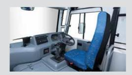
4-way Adjustable Driver Seat, provides complete head & back support to driver with 3 Point ELR Type Driver Seat Belt
