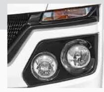
Twin Round Headlamps provide better light spread at night with both upper and dipper light arrangement for better light vision & safer night driving for drivers
