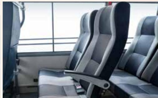
Ergonomically Designed Lumbar and Head Support. 295 mm Roomy Legroom. Wide Seat Pitch - 680 mm. Maximum Seat Depth - 415 mm
