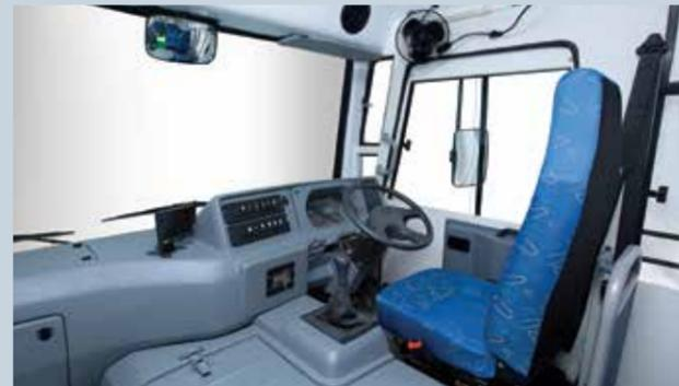
4-way Adjustable Driver Seat, Inbuilt Headrest, 3-point Emergency Locking Retractor Type Driver Seat Belt
