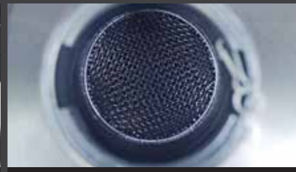
Wire Mesh for Fuel Theft Protection
