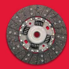
Both the FURIO 7 HD and the FURIO 7 Tipper come with an LUK Clutch; of 280 mm and 310 mm diameters respectively. The bigger diameter provides more contact area and better power transmission without any slippage. There's even a booster to lower the effort of clutch operation and higher lining life to lower maintenance cost. What's more, there's a wear-indicator to let you know when you need to replace it.
