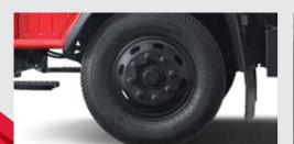
Tubeless and Radial Tyres\* for High Speed Capacity, Better Stability And Puncture Resistance
