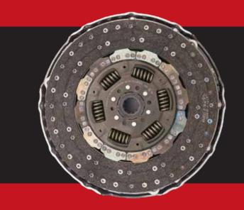
When it comes to the clutch, you'll see the same design philosophy. A bigger, 362 mm diameter organic clutch provides more contact area and better power transmission without slippage. It comes with a booster that leads to lower effort in clutch operation. The LUK B 8090 clutch also has a higher lining life which translates to lower maintenance cost. And the best aspect of this clutch is the wear indicator that lets you know when it is time to replace it.
