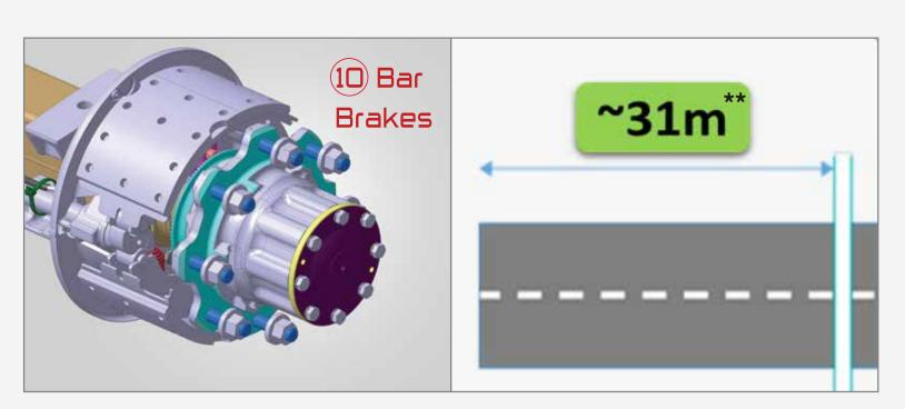
10 Bar Braking System for Quick, Short Stops
