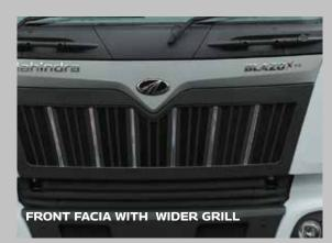
Wide spaced grills so air can enter easily and cool the radiator at all times
