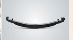
Softer Parabolic Suspension with Rubber Tips for Best-In-Class Comfort to Absorb Bumps and Jerks
