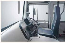
4-way Adjustable and Fully Reclining Driver's Seat Tilt and Telescopic Steering
