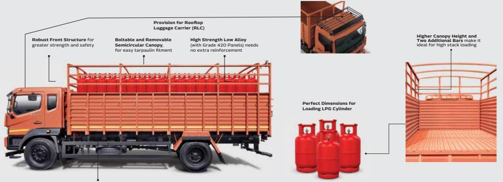
Dense Pitch Side Pillars offer better load support and prevent panel deformation
