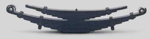
The suspension of the Mahindra FURIO follows the classic Mahindra reliability in its design and build. This rear, semi-elliptical suspension is **heavy duty** and has the capability to take on the toughest driving and load conditions **without any need for additional leaves**.
