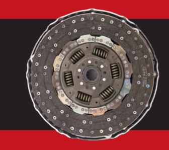
When it comes to the clutch, you'll see the same design philosophy. A **bigger**, **362 mm diameter organic clutch** provides more contact area and better power transmission without slippage. It comes with a **booster** that leads to lower effort in clutch operation. The LUK B 8090 clutch also has a **higher lining life** which translates to **lower maintenance cost**. And the best aspect of this clutch is the **wear indicator** that lets you know when it is time to replace it.
