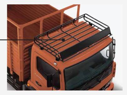
**Robust Front Structure** for greater strength and safety **Boltable and Removable Semicircular Canopy,** for easy tarpaulin fitment High Strength Low Alloy (with Grade 420 Panels) needs no extra reinforcement
