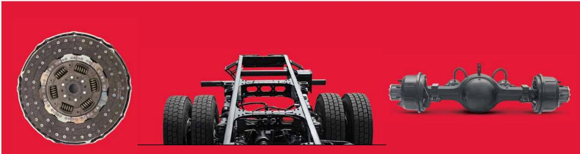
362 mm Diameter Organic Clutch High Strength Low Alloy Material (HSLA 550) Heavy-Duty Rear Axle Meritor
