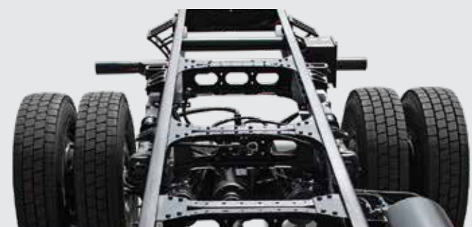
High Strength Low Alloy Material (HSLA 550)
