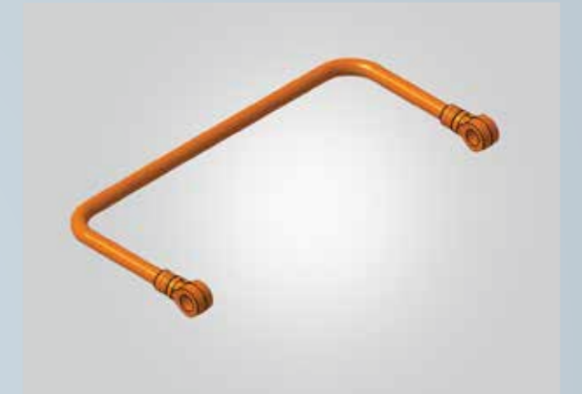
Anti-Roll Bar for Stability at High Speed
