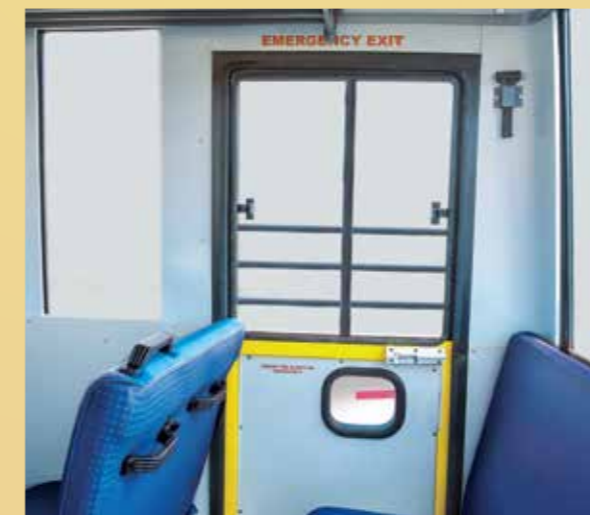
Emergency Exit for Quick Evacuation in Case of Exigency
