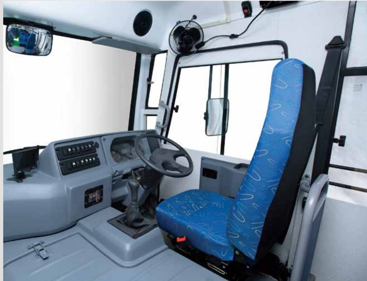
4-way Adjustable Driver Seat, Inbuilt Headrest, 3-point Emergency Locking Retractor Type Driver Seat Belt
