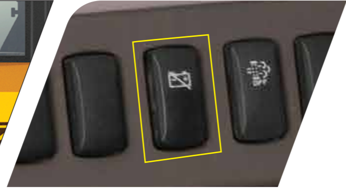
Electronically Operated Battery Switch With Auto Cut-Off
