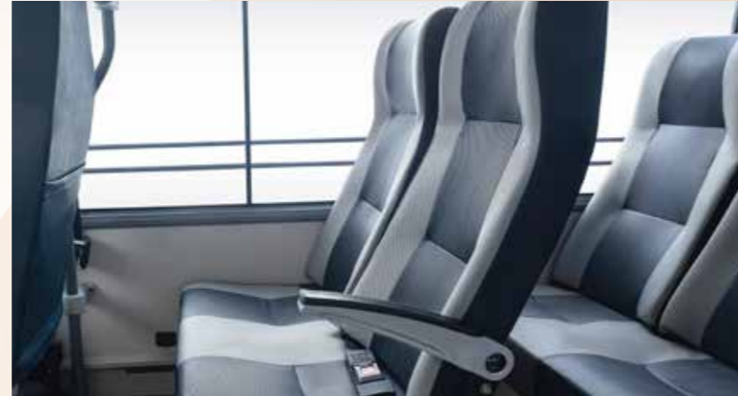
Ergonomically Designed Lumbar and Head Support. 295 mm Roomy Legroom. Wide Seat Pitch - 680 mm. Maximum Seat Depth - 415 mm
