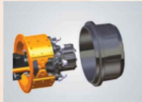
Biggest Brake Liners (325 mm x 155 mm) for Reduced Stopping Distance
